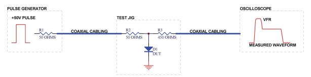
The pulse generator (an AV-1010-B, in Avtech's tests) generates +50V pulses with < 10 ns rise and fall times. The output impedance of the pulser is set to 50 Ohms, and a 50 Ohm resistance is in series with the DUT, so the pulsed current is (50V / 100 Ohms) = 500 mA. The 450 Ohms in the output branch is terminated by an oscilloscope with 50 Ohm input impedance, so that the oscilloscope displays  $V_{DUT} / 10$ .
