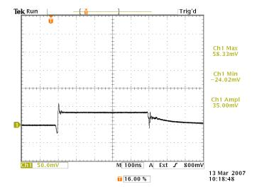
A small inductive spike is observed on both edges of the waveform. Most of this spike is due to the internal device inductance, and is thus "real" and needs to be included in  $V_{\text{FR}}$  measurements.
