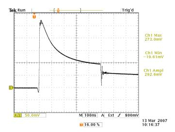
The MUR8100E is very slow to turn on – the turn-on transient has not actually finished in the above waveform before the input pulse ends.
