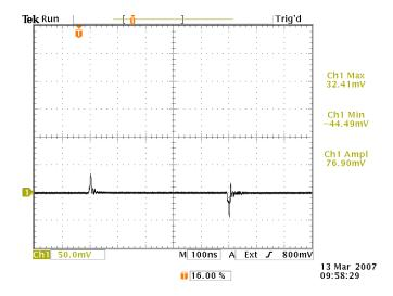
This waveform is scaled at 50 mV/div and 100 ns/div, the same as the user's waveform on the previous page. The inductive spike is approximately 35 mV  $\times$  10 = 350 mV, about one-quarter of that observed before. This corresponds to  $\sim$  7 nH of inductance, most of which comes from the shorting wire itself.
