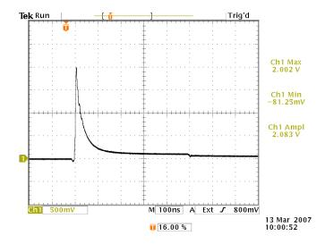
In this test,  $V_{FR}$  reaches 20V (2.002V × 10), compared to 0.58V for the 1N5819! In this case, the inductance of the original test jig would not have been noticed, because the inductive voltage was far smaller than the voltage generated by the PN junction itself.
