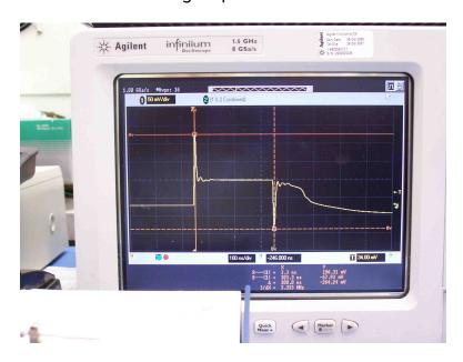
The user was concerned about the large spikes on the rise and falling edges. To determine if these were caused by the device action itself, or by parasitic inductance, the user replaced the DUT with a short circuit (a small piece of wire). The resulting waveform showed the same spikes:
