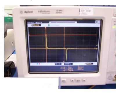
This clearly shows that the spikes are inductive in nature. The rising-edge spike is equal and opposite to the falling-edge spike, as one would expect for an inductor. The parasitic inductance can be estimated from the amplitude of the spikes ( $V \approx 1.4V$ ), the current ( $dI \approx 500$  mA), and the rise time ( $dt \approx 10$  ns):  $V = L \times dI / dt$ , so  $L \approx 28$  nH.
