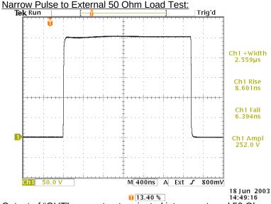
Output of "OUT" connector, terminated into an external 50 Ohm load. Viewed with TDS3052 scope. 50V/div, 400 ns/div.
