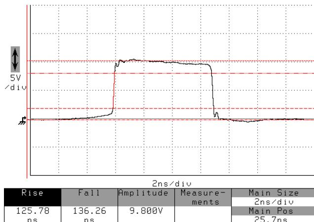
The AVMP series of pulse generators offer 10V or 20V outputs with sub-nanosecond rise times, and pulse widths variable from several nanoseconds up to 100 ns, 1 us, or 10 us.
