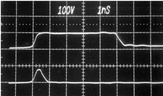
AVR-E4-B-P, at maximum & minimum pulse widths.
