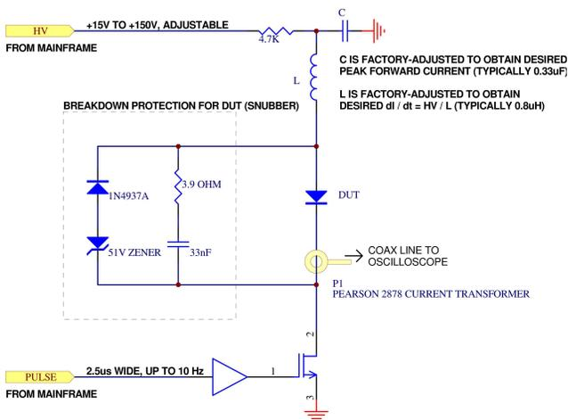
This approach uses a DC-biased MOSFET (with intrinsic body diode) as the switching element, rather than the AC-biased SCR approach shown in MIL-STD-750-4 Figure 4031-6. This is not expected to affect the results in any significant way.
