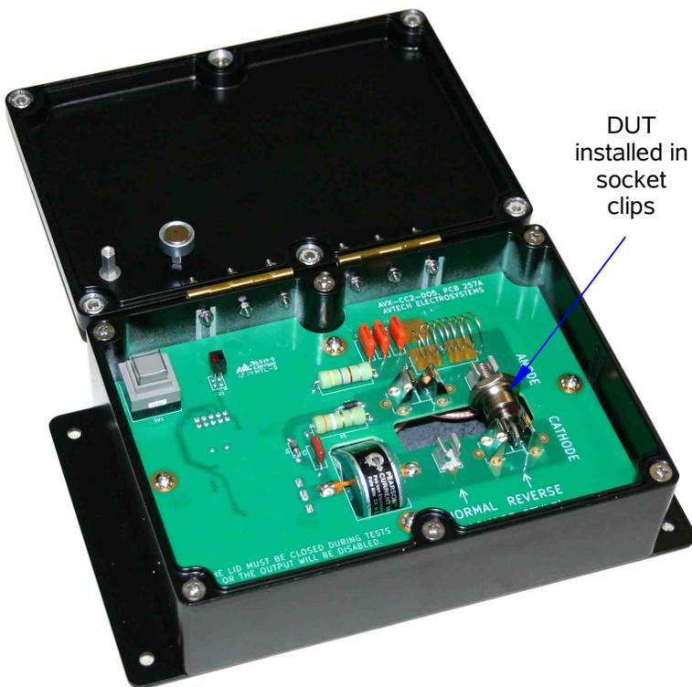
A typical test jig is shown at the left, with clip socketing for normal and reverse-polarity DO-5 stud packages. Test jigs are normally customized to meet specific customer requirements.
