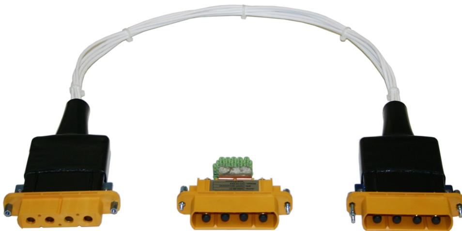
*AK9 kit, including the AV-HLZ1-100 output cable (right and left) and mating adapter (middle). The adapter is shown with some test resistors installed on copper brackets. The copper brackets are screwed into the four contact posts on the rear of the adapter. These brackets and resistors are not included with the adapter; this is just a sample configuration.*
