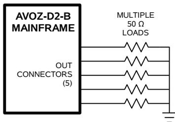
When used to drive loads with impedances less than 50 Ohms, two or more outputs can be combined at the load in an optional output module:
