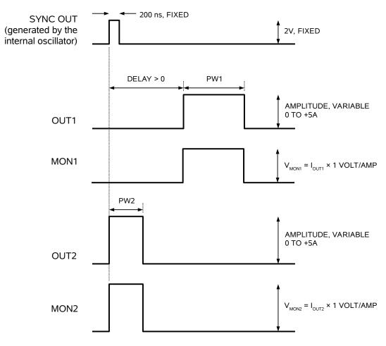
Basic Output Pulses for Delay > 0
