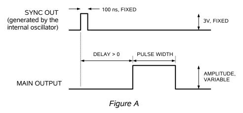
If the delay is negative, the order of the SYNC and OUT pulses is reversed:
