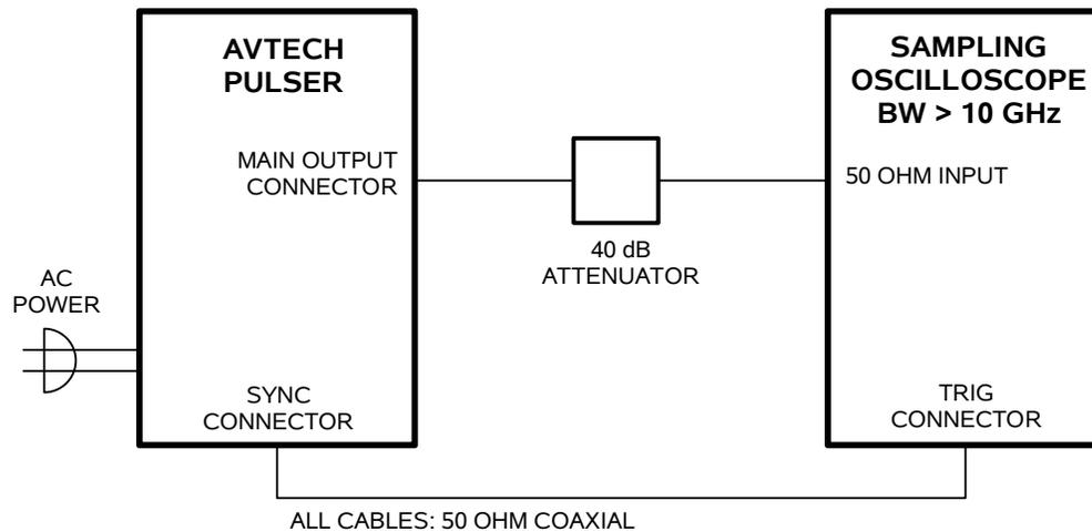
1. Connect the pulse generator to a sampling oscilloscope as shown above. Note that:
