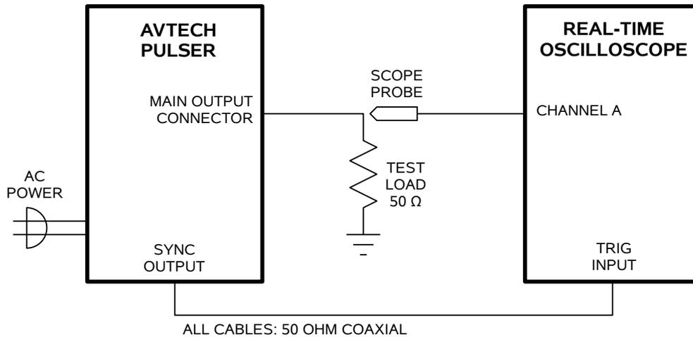
*BASIC TEST ARRANGEMENT, WITH A REAL-TIME OSCILLOSCOPE*
