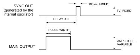
Basic Output Pulses for Delay < 0
