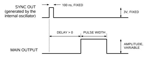
Basic Output Pulses for Delay > 0
