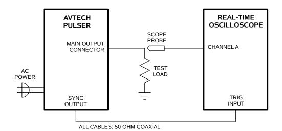
1. Connect a cable from the SYNC OUT connector to the TRIG input of an oscilloscope. Connect the AV-HLZA1 test load directly to the rear-panel OUT connector and place the scope probe across this load. The probe signal clip should be attached to the narrow copper strip, and the ground clip should be attached to the wide copper strip. If you intend to operate at high duty cycles, the test load should be fan-cooled to dissipate the maximum possible 10 W of heat.
