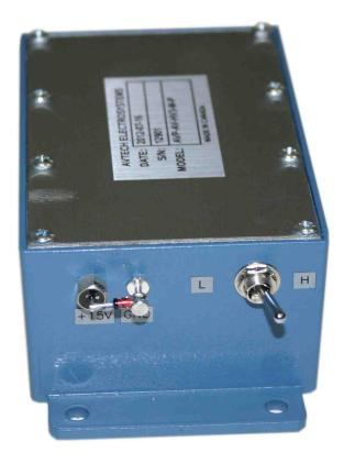
The +15V input terminal is protected with a 1N4746A Zener diode, which will fail as a short if an excessive positive voltage (> 18V), or a negative voltage, is applied to the terminal.
