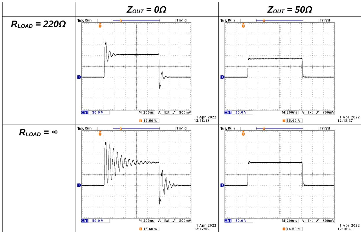
It should be observed that maximum voltages are obtained when  $Z_{OUT} = 0\Omega$ , but transmission line reflections are minimized with  $Z_{OUT} = 50\Omega$ . Also, regardless of the value of  $Z_{OUT}$ , reflections and ringing are minimized when  $R_{LOAD} = 50\Omega$ .
