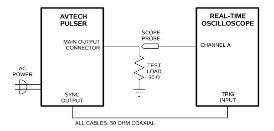
BASIC TEST ARRANGEMENT, WITH A REAL-TIME OSCILLOSCOPE
