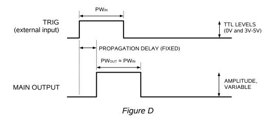
The delay, pulse width, and frequency (when in the internal mode), of the OUT pulse can be varied with front panel controls or via the GPIB or RS-232 computer interfaces.
