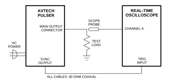
1. Connect a cable from the SYNC OUT connector to the TRIG input of an oscilloscope. Connect a 100 k $\Omega$  (or higher) load to the OUT connector and place the scope probe across this load. The load resistor <u>must</u> have a voltage rating of at least 400V. The power dissipated in the resistor is given by
