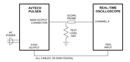
BASIC TEST ARRANGEMENT, WITH A REAL-TIME OSCILLOSCOPE
