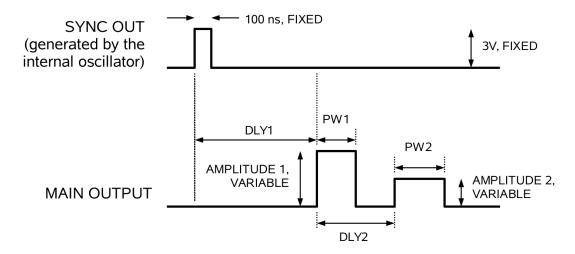
PW1, PW2, DLY1, DLY2, AMPLITUDE 1 and AMPLITUDE 2 are adjustable settings.
