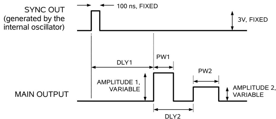
PW1, PW2, DLY1, DLY2, AMPLITUDE 1 and AMPLITUDE 2 are adjustable settings.
