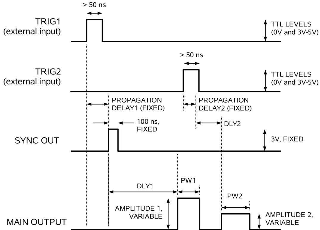
A 50 Ohm load is *required* for proper operation. The output stage may be damaged if the output is not terminated into a 50 $\Omega$  load.
