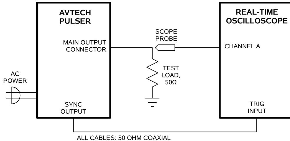
*BASIC TEST ARRANGEMENT, WITH A REAL-TIME OSCILLOSCOPE*
