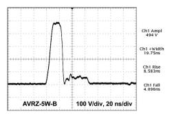
This transient should be less than 20% of the peak amplitude, and less than 100 ns in duration.
