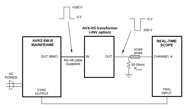
The transformer is capable of operating up to the maximum rated pulse width of the AVRZ-5W-B (10 us). The transformer may introduce slight rounding and ringing to the output waveform, and it may degrade rise and fall times slightly (by 1-3 ns, typically). A typical waveform photo is shown below:
