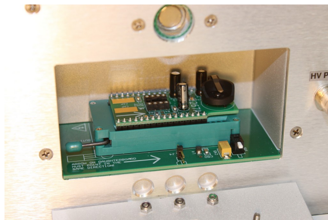
Daughterboard installed in ZIF socket, in positive position
