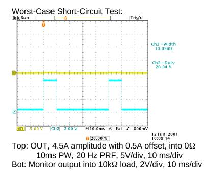
a) Output Signal Amplitude: 0-5A
