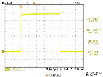
+100A into  $0.96\Omega$ , maximum pulse width and duty cycle
