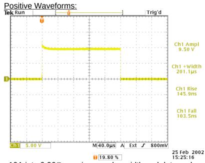
+10A into  $0.96\Omega$ , maximum pulse width and duty cycle
