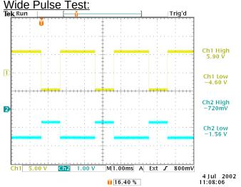
Top: OUT, -10V with +6V offset, 1 ms PW, into 50  $\Omega$  5V/div, 1 ms/div
