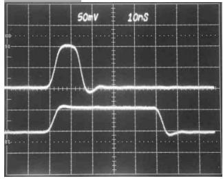
Top: +10V into  $50\Omega$ , minimum pulse width (15 ns)
