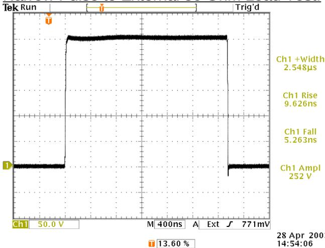
Output of "OUT" connector, terminated into an external 50 Ohm load. Viewed with TDS3052 scope. 50V/div, 400 ns/div.
