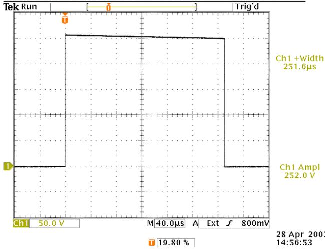
Output of "OUT" connector, terminated into an external 50 Ohm load. Viewed with TDS3052 scope. 50V/div, 40 us/div.
