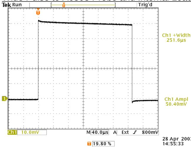
Output of A6303 probe, viewed with TDS3052 scope. The A6303 probe is clamped to the shorting bar.
