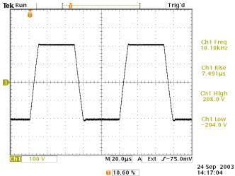
Square wave output into a load consisting of 5000 Ohms and 10000 pF in parallel. 10 kHz. 20 us / div, 100 V/div.
