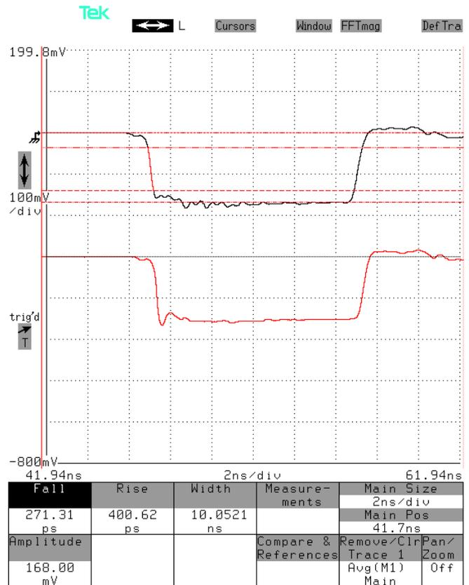
Bottom: “MI” output. 2V/div (200 mV/div × 20 dB). This shows that the pulse amplitude after the inverting transformer is  $-3.1V \times 11 = -34V$ , approximately. (There is ~21% loss in the transformer).
