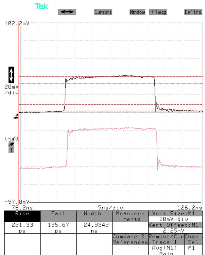
Top: Voltage measured across the resistor in response to a +4.7V pulse applied from an Avtech AV-1030-C pulse generator. It should be approximately  $(+4.7V / 54.6\Omega) \times 4.6\Omega = 396\text{ mV}$ , which agrees with the observed waveform. 200 mV/div (= 20 mV/div × 20 dB), 5 ns/div.
