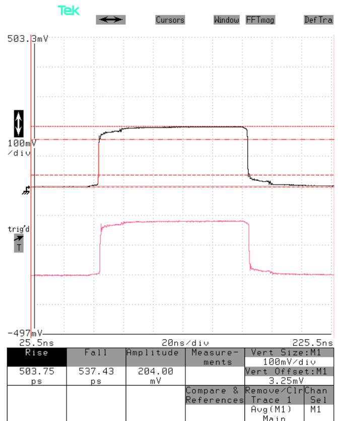
Top: Voltage measured across the resistor in response to a +4V pulse applied from an Avtech AV-1030-B pulse generator. It should be approximately  $(+4V / 50\Omega) \times 25\Omega = +2V$ , which agrees with the observed waveform.
