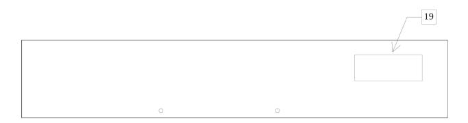
19. AC POWER INPUT. A three-pronged recessed male connector is provided on the back panel for AC power connection to the instrument. Also contained in this assembly is a slow blow fuse and a removable card that can be removed and repositioned to switch between 120V AC in and 240V AC in.
