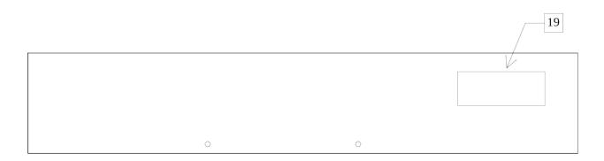
19. AC POWER INPUT. A three-pronged recessed male connector is provided on the back panel for AC power connection to the instrument. Also contained in this assembly is a slow blow fuse and a removable card that can be removed and repositioned to switch between 120V AC in and 240V AC in.
