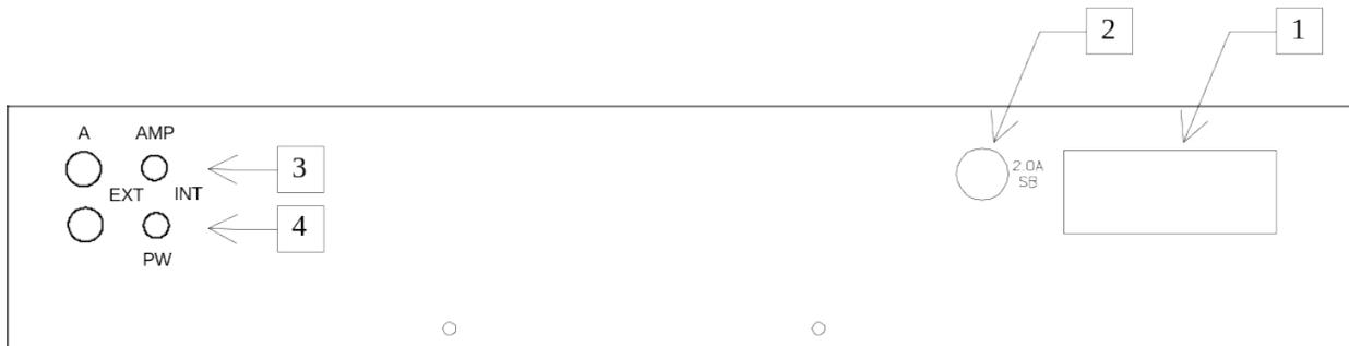
1. AC POWER INPUT. A three-pronged recessed male connector is provided on the back panel for AC power connection to the instrument. Also contained in this assembly is a 1.0A slow blow fuse and a removable card that can be removed and repositioned to switch between 120V AC in and 240V AC in.
