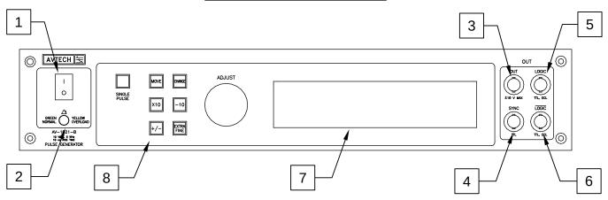
1. <u>POWER Switch</u>. This is the main power switch. When turning the instrument on, there is normally a delay of 10 seconds before anything is shown on the main display, as the internal operating system boots up.
