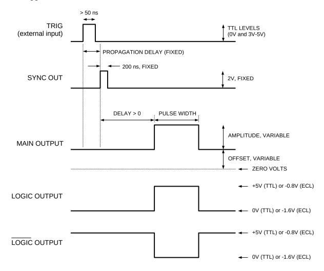
As before, if the delay is negative, the order of the SYNC and OUT pulses is reversed.
