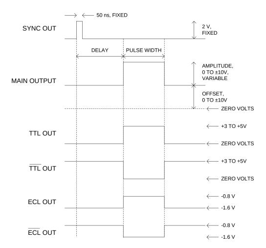
The next figure illustrates the relationship between the signals when an external TTL-level trigger is used (i.e., the REPETITION RATE switch is set to "EXT"):
