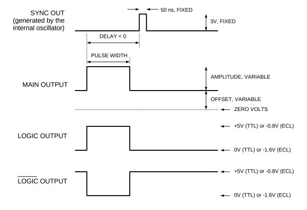
The next figure illustrates the relationship between the signals when an external TTL-level trigger is used:
