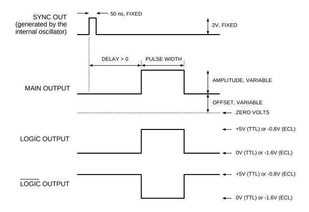
If the delay is negative, the order of the SYNC and OUT pulses is reversed:
