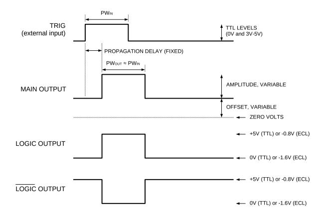
The delay, pulse width, and frequency (when in the internal mode), of the OUT pulse can be varied with front panel controls or via the GPIB or RS-232 computer interfaces.
