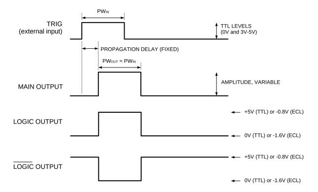
The delay, pulse width, and frequency (when in the internal mode), of the OUT pulse can be varied with front panel controls or via the GPIB or RS-232 computer interfaces.
