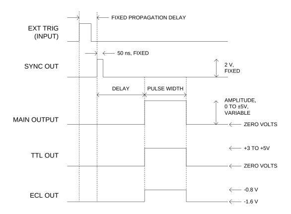
As before, if the delay mode is set to "MAIN OUT ADVANCED", the order of the SYNC and OUT pulses is reversed.
