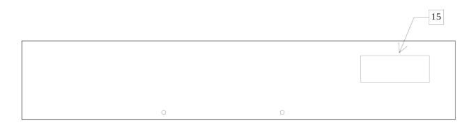
15. AC POWER INPUT. A three-pronged recessed male connector is provided on the back panel for AC power connection to the instrument. Also contained in this assembly is a slow blow fuse and a removable card that can be removed and repositioned to switch between 120V AC in and 240V AC in.
