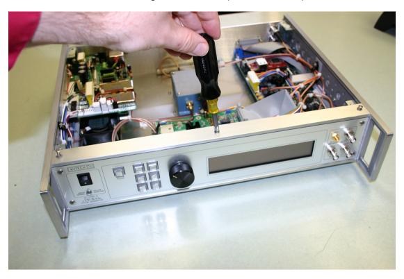
21. Re-install the top cover, by sliding it on from the rear, and installing the four cover screws.
