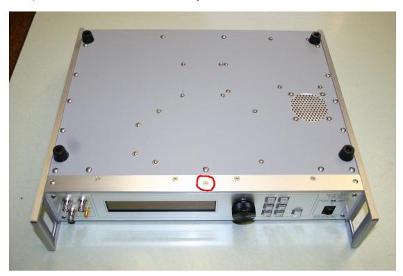
5. Flip the instrument over, right side up. There is a screw in each of the four corners of the front panel. Remove these. The front panel is now unsupported. Gently pull it forwards to permit easier access to the back side of the front panel.
