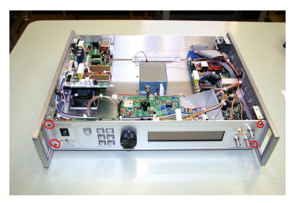
6. Three BNC cables and one SMA cable must be disconnected from the bulkhead connectors behind the "OUT" area of the front panel. Keep track of where each of the three BNC connectors is supposed to go. (The upper-most BNC cable has a black strain relief. The lower two do not.) The BNC cables can be disconnected from the front-panel bulkhead connectors by hand. The SMA cable needs to be disconnected using a small wrench.
