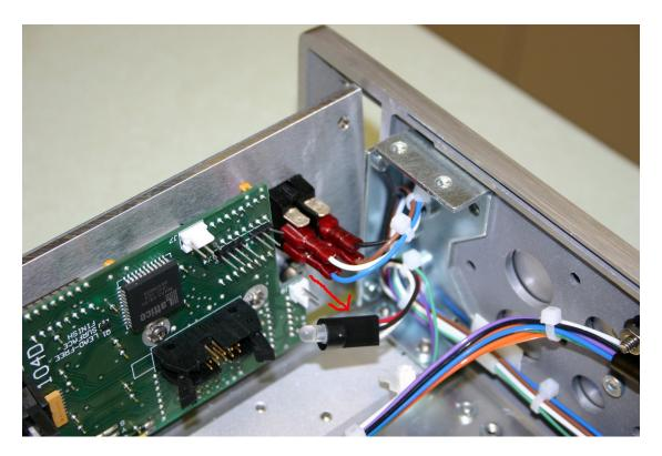
10. Lastly, use pliers to disconnect the four wires (black, white, blue, brown) from the power switch.
