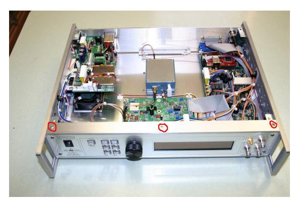
4. Flip the instrument over, upside down. Three screws secure the bottom crossbar before the front panel. Remove the middle screw only.
