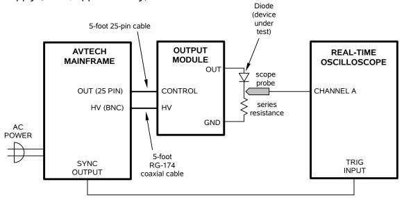
The diode is shown oriented for positive (-P) operation. It must be reverse for negative (-N)
