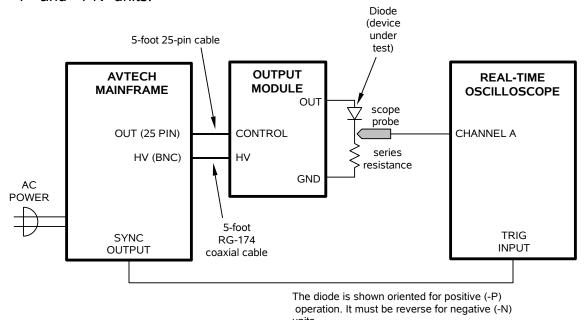
For negative units (or negative use of dual-polarity units), the diode must be reversed.
