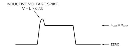
Attaching a current transformer (for measuring current waveforms) can add significant inductance, because of the necessary wire length that must be fed through the transformer. The Pearson 2878 requires approximately 1.5", and the 410 requires 3". Both will degrade the output current rise time.
