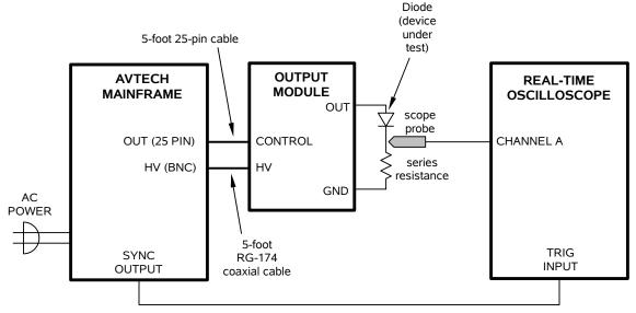
The diode is shown oriented for positive (-P) operation. It must be reverse for negative (-N) units.
