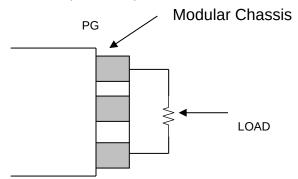
Take care to insure that during soldering the OUT conductor is not shorted to the chassis. Also, use minimal heat when soldering.
