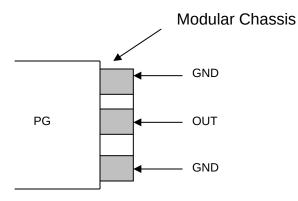
The load should be connected between the OUT and GND terminals using very short leads ( $\leq 0.5$  cm).
