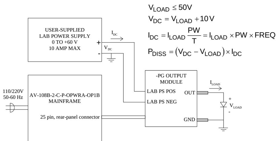
The AV-108B-2-C-P-OPWRA-OP1B includes provision for water-cooling, which should be used when the power dissipated in the output module ( $P_{DISS}$ ) exceeds 30 Watts.
