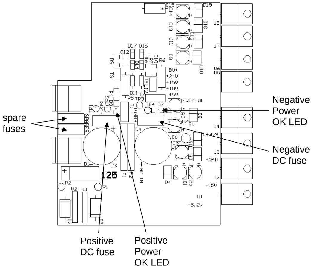
The positive fuse and one of the spare fuses on this circuit board are 1A slow-blow fuses, Littlefuse part number R452001. (This fuse can be ordered from Digikey, [www.digikey.com](http://www.digikey.com). The Digikey part number is F1343CT-ND). The negative fuse and the second spare fuse are 0.5A slow-blow fuses (Littlefuse R452.500, Digikey part number F1341CT-ND).
