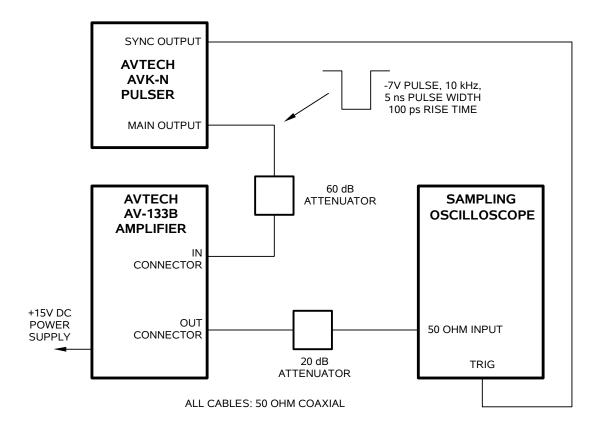
The factory test set-up is shown above.
