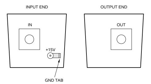
The input and output SMA connectors are located on opposite ends of the module, as shown above.
