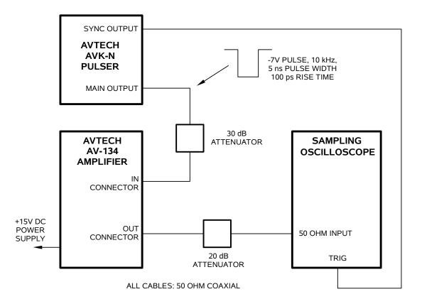
The factory test set-up is shown above.
