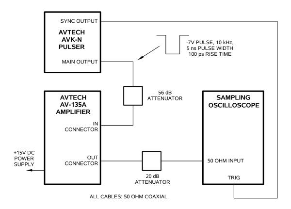
The factory test set-up is shown above.
