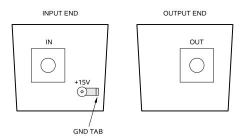
The input and output SMA connectors are located on opposite ends of the module, as shown above.
