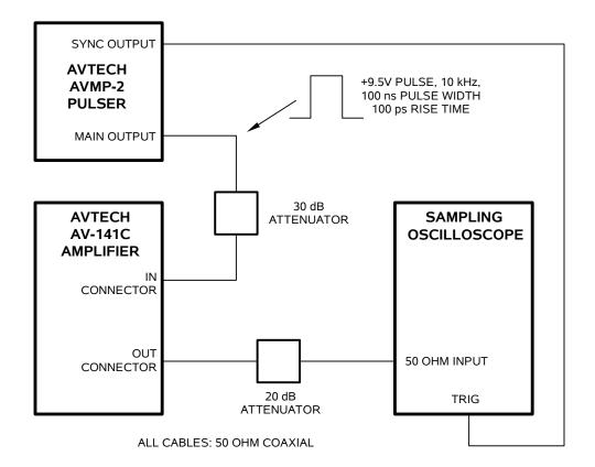
The recommended test set-up is shown above.
