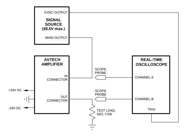
The recommended test set-up is shown above. The Avtech AV-1030-C pulse generator is a suitable signal source.
