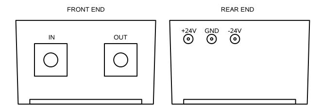
The input and output SMA connectors are located on the front end of the module, as shown above. The +24V, -24V, and GND input solder terminals are located on the opposite end.
